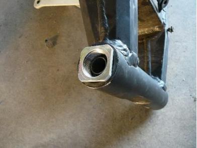
Once your swing arm fits, fabricating the swing arm pivot tube sleeve...
