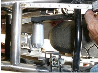
Insert piping, make sure you have enough clearance from shock springs to pivot tube and tack weld your shock support to t support. Don't tack to the frame yet, we'll remove and give it a good weld first then install back on for the frame welds.
