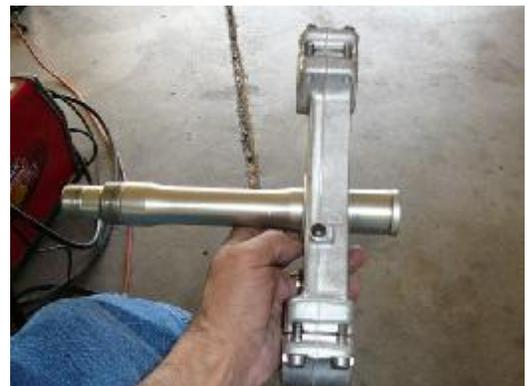
Lucky for me, I have a metal manufacturer we have used in business for the last 8 years so I got a freebie on the triple tree sleeve. Basically 37.5mm in height, 36mm in width where the whole opening is the same as the KZ900 steering stem.
