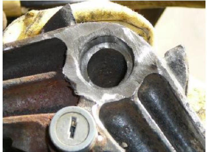
Now onto the removal of the ZX steering stem from the lower triple tree. I tried everything possible with heat and a 6 ton press. I searched for an answer and came up with nada, and even posted a question on the forum, still no answer for which way did this stem press out...
