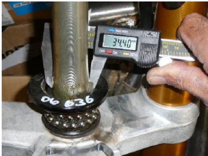
Well then, no use in panicking for the only solution I had was to remove the KZ900 steering stem and press it into the ZX636 lower triple tree. Seemed easy enough but I had no idea what I was getting into for I was determined... LOL!
