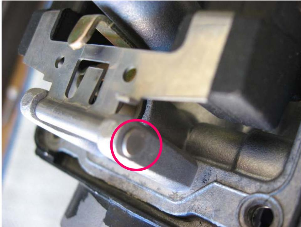
Float pin has a nail-head detail on one end and round on the other
