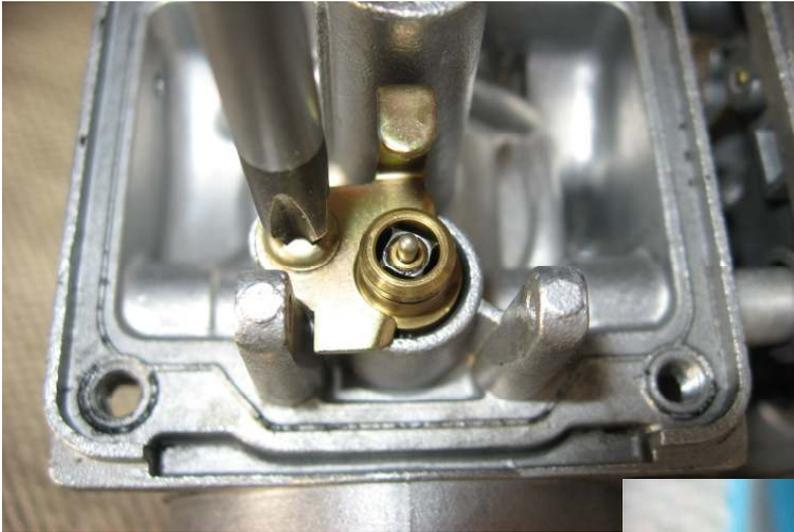
Inspect the float needle and seat carefully. The spring on the needle must be smooth and the tip free of wear (if you feel a ridge on the tapered portion of the needle it needs to be replaced).
