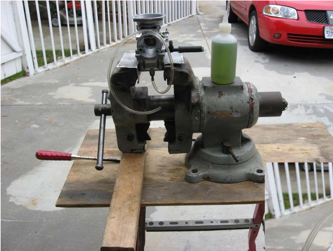
Feed fuel in until the float stops the flow. An elevated reservoir is recommended (works better than bottle as shown)
