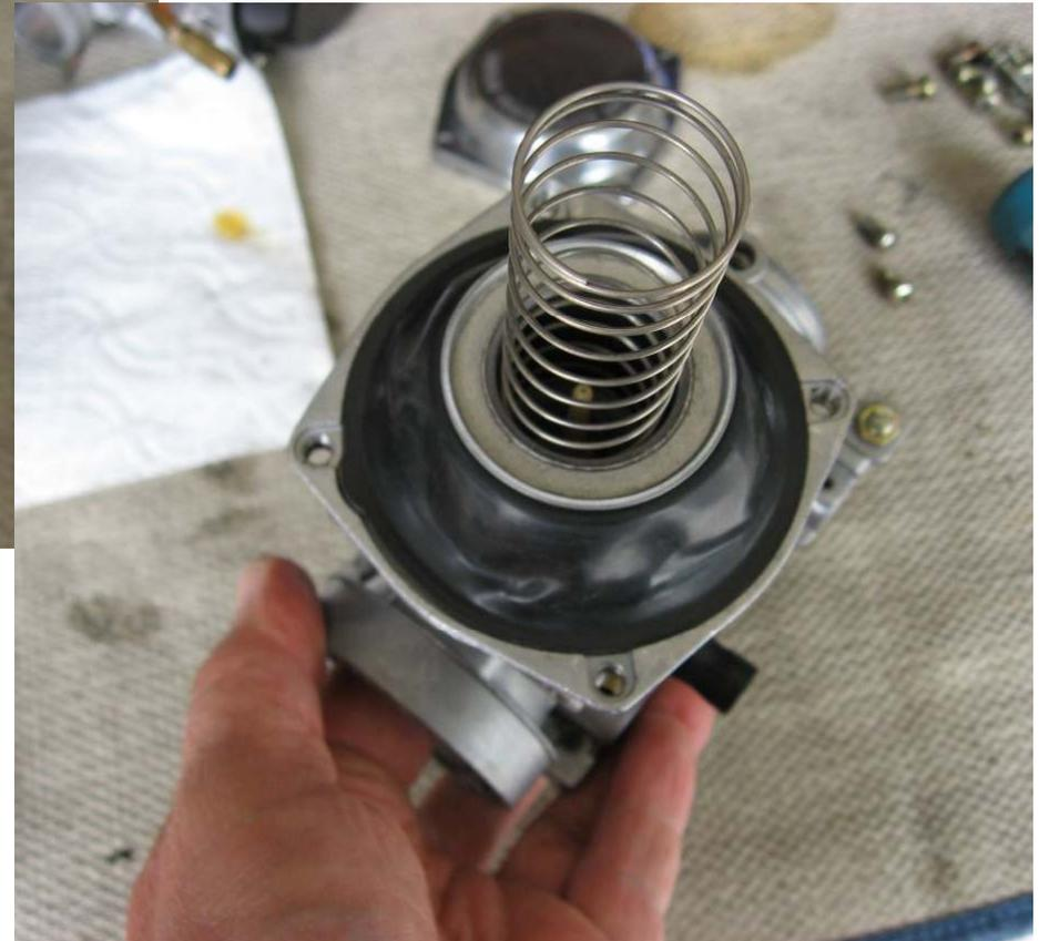
Hold up slide with finger then install cap
