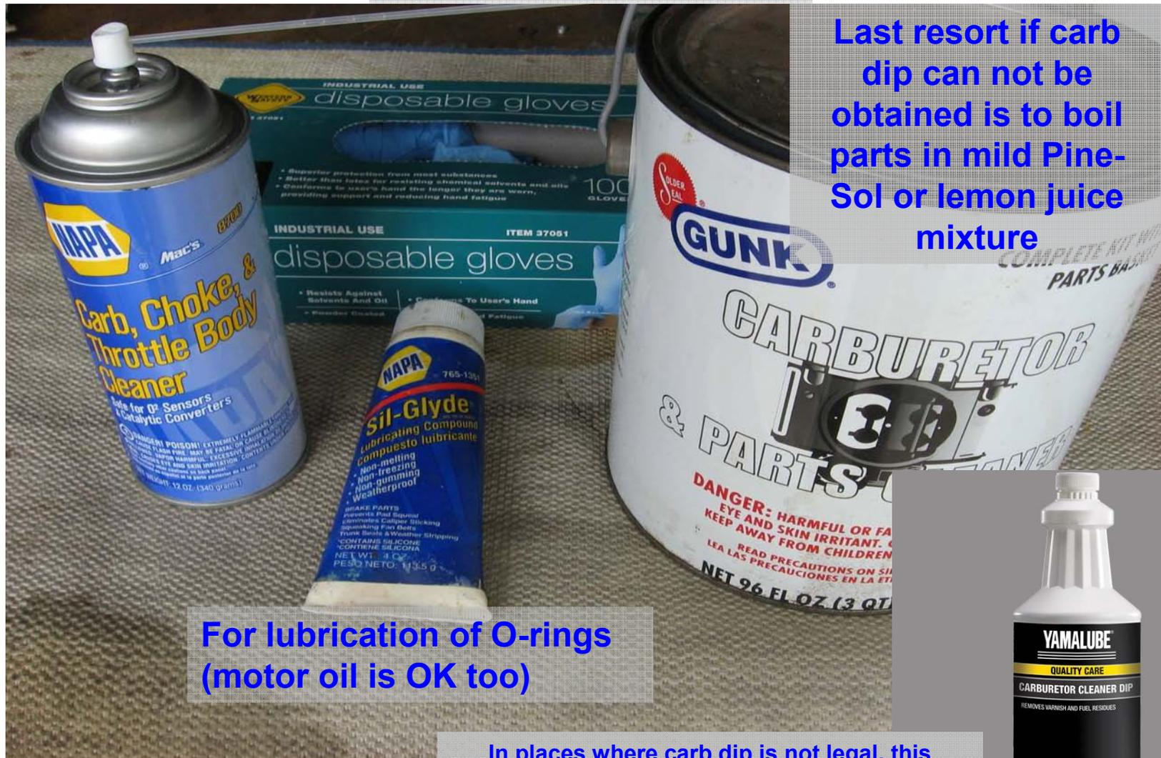
Last resort if carb dip can not be obtained is to boil parts in mild Pine-Sol or lemon juice mixture
