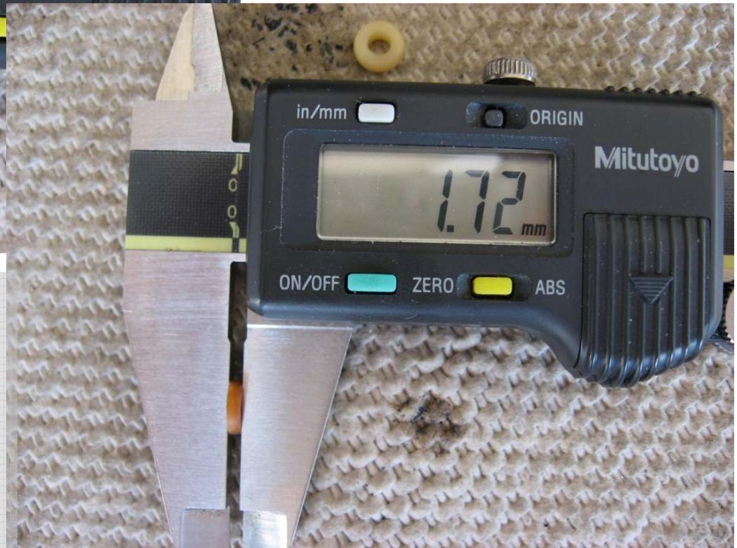
Reducing the thickness of the plastic spacer on top of the needle clip results in a richer mixture. Old plastic spacer can be sanded down or replaced with a washer stack thinner than original spacer.
