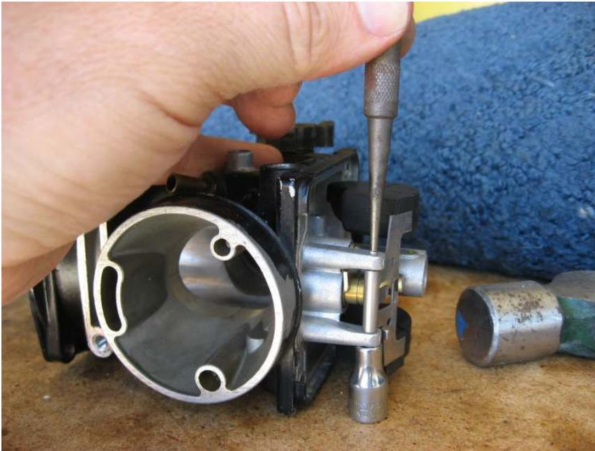
Gently tap the drift to remove the pin. **CAUTION: Do NOT use a lot of force or the float post will snap off.**
