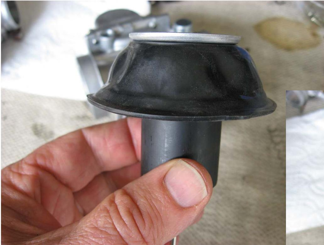
Forming the diaphragm in this way makes it easier to keep the lip in the groove on top of the carbs while installing top cap.
