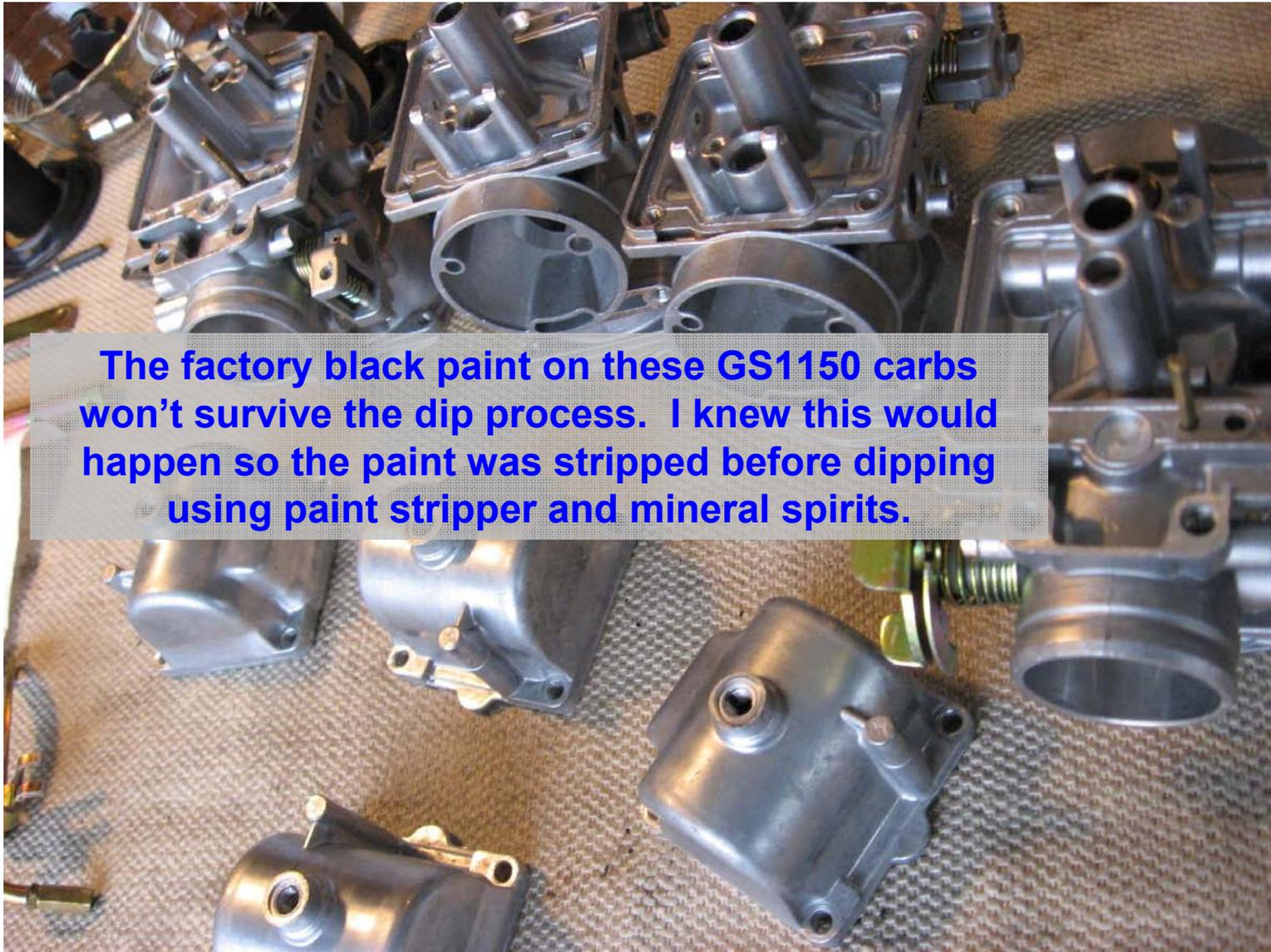
The factory black paint on these GS1150 carbs won't survive the dip process. I knew this would happen so the paint was stripped before dipping using paint stripper and mineral spirits.
