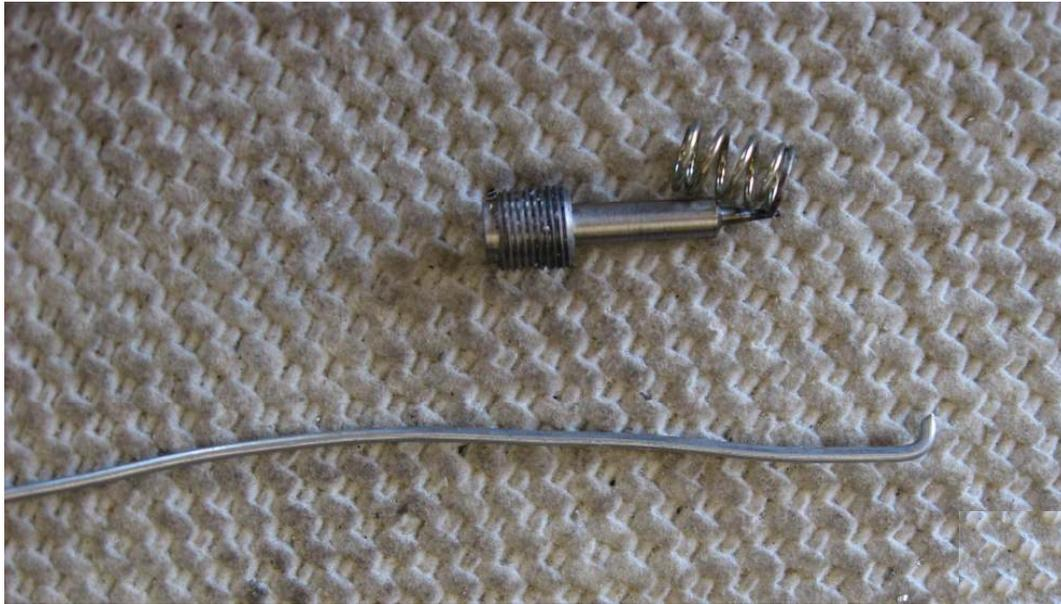
O-ring and washer often hang up inside the carb body and must be extracted from down in pilot screw tunnel
