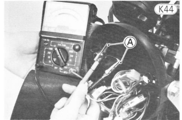
A. Brake Light Switch Leads
