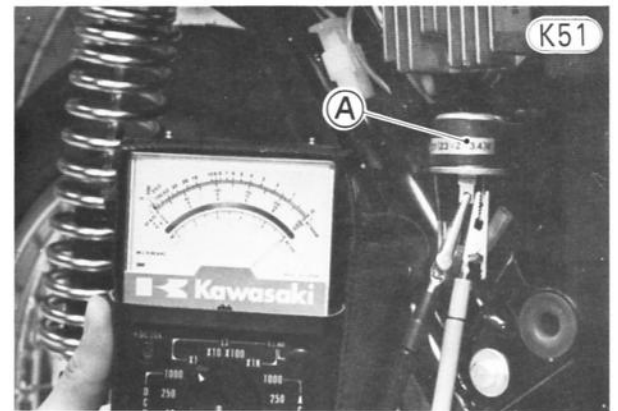
A. Turn Signal Relay
