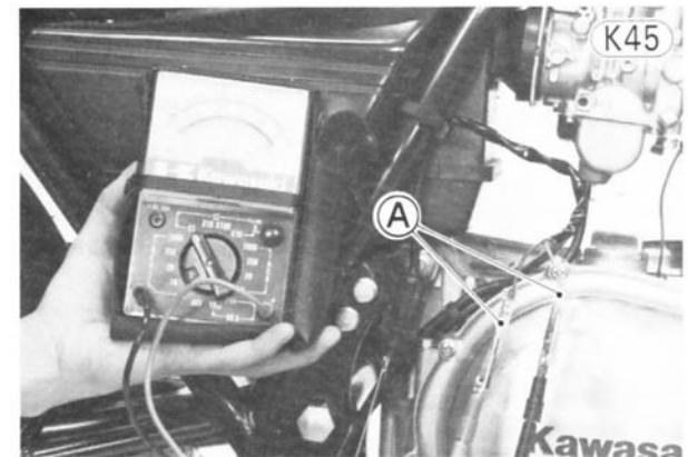
A. Brake Light Switch Leads
